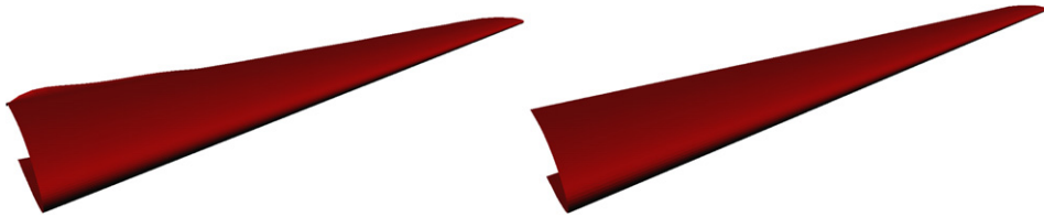
Fig. 8. Left: The initial parametrization of the front of a Falcon airplane. Right: The final parametrization after trimming procedures were applied to the figure on the left.
